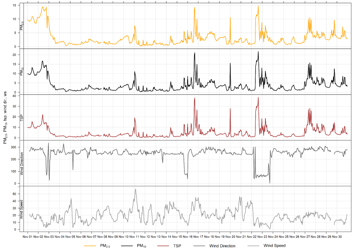
Figure 5-1 1-hour particulate matter concentrations at the West monitor
